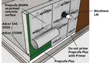
Preprufe 800PA post-applied to walls in conjunction with Preprufe Plus below slabs
