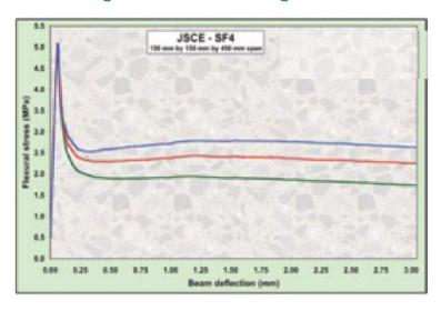
Note: These curves are based on averages of several beam tests. The toughness performance will depend on the concrete mix design used.
