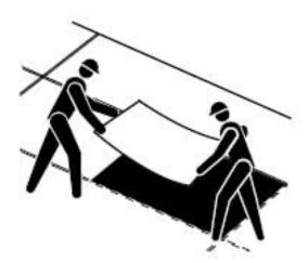
Where protection abut the parapet, pipe bays or abutments they should be pre-measured, and accurately cut to size by incising with a sharp knife and breaking on edge. The joints between the protection/membranes should be dry.
