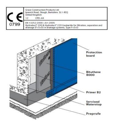
Details shown are typical illustrations only and not working drawings. For assistance with working drawings and additional technical advice please contact GCP Technical Services.
