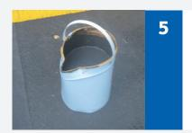
Squeeze the sides of the tin together to form a spout to aid pouring into the draw box.
