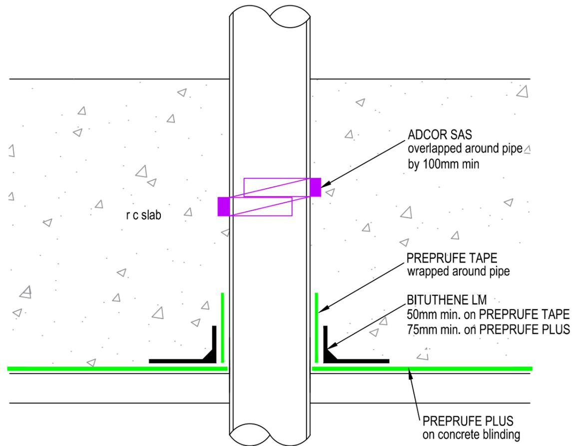
**PIPE THROUGH RC SLAB SECTION**
