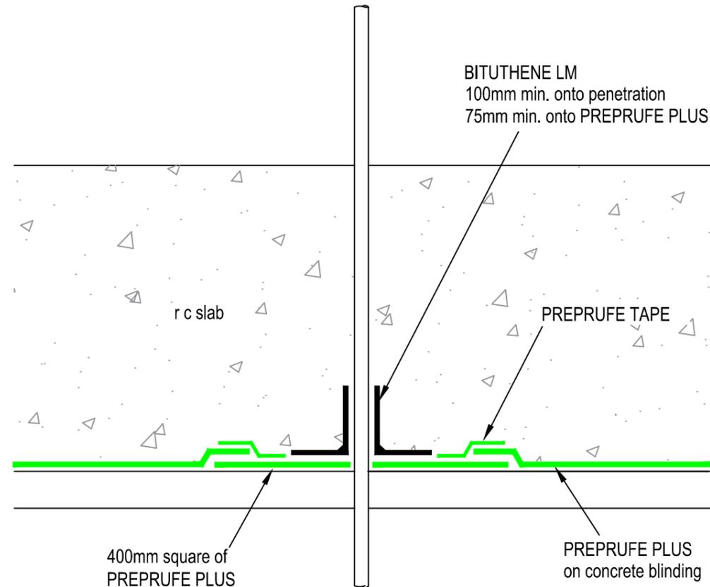
**RC SLAB - ROD PENETRATION SECTION**
